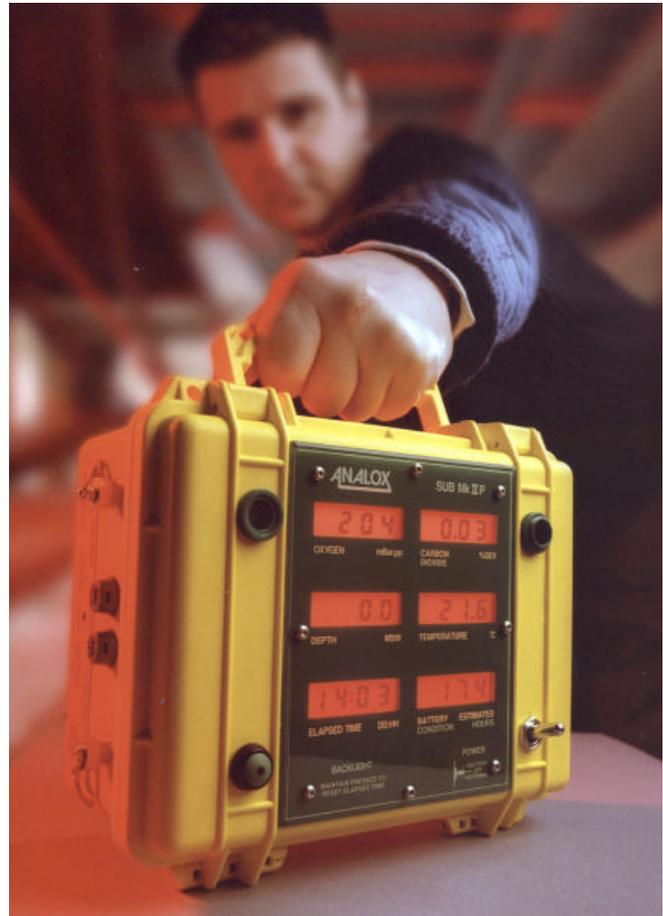
**The Sub MKIIP™ is specifically designed for operation in a DISSUB scenario**
